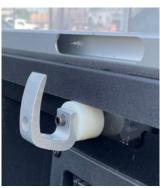
2. Insert the M6 bolt into the clamp base. Use 2 each 1/2" plastic spacers between the clamp base and the vehicle. Tighten the clamp base to the vehicle with a 4.5mm Hex Key. DO NOT OVER TIGHTEN.
