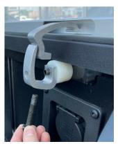
3. Install the upper clamp into the side rail slot. Insert the 3/8" flange head bolt through the bottom of the base clamp and tread into the upper clamp.
