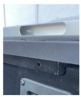
1. Locate the mounting hole that aligns with the center of the side rail slot.
