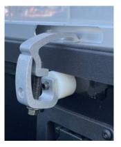
4. With the 14mm wrench, tighten the flange head bolt to secure the side rail to the vehicle. DO NOT OVER TIGHTEN.
